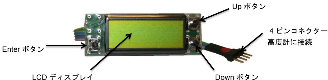
図 1. The RC Electronics Programming Card
